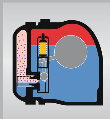
Condensate discharge without the presence of air (temperature at saturation temperature).
