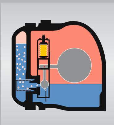
Air-venting during operation (temperature below saturation temperature).
