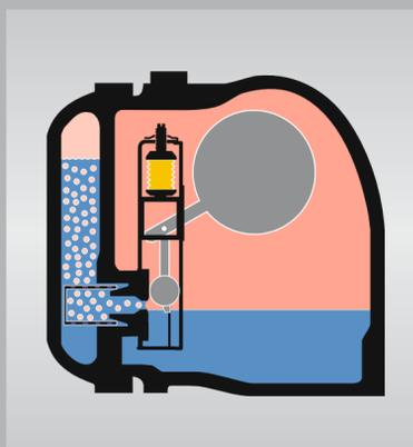
Air-venting with the plant cold (during start-up). Thermostatic bellows lifts up the ball float.
